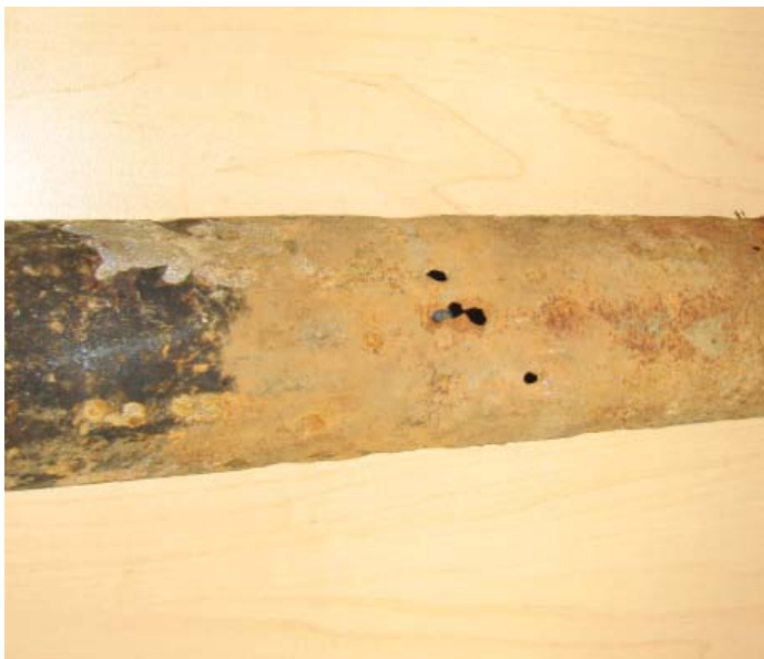
Section of gas pipe recently replaced
